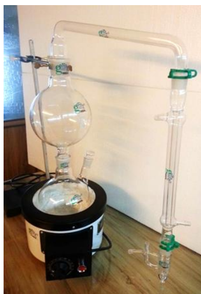
Plate 1. An assemblage of clevenger apparatus used for oil extraction through hydrodistillation process
