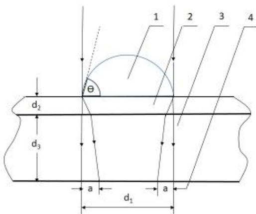
**Fig. 1. Operation principle of the method for measurement of the wetting angle of liquid drops on a hard surface**
