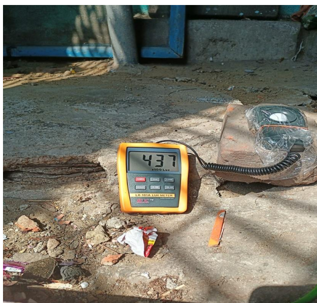
Fig. 6. Light Sensor of the “LUX METER” placed outside the septic tank. Reading is :- 437 x100 = ‘43,700’Lux (Time - 10 AM)
