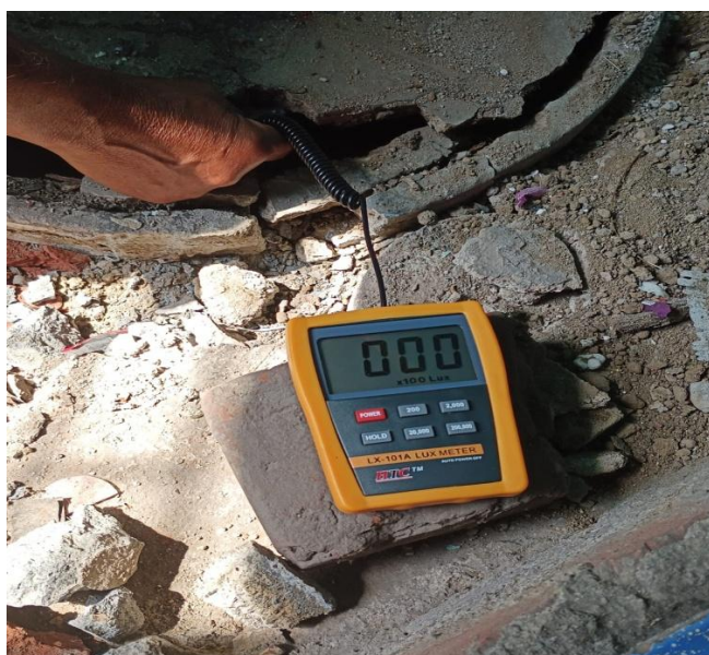
Fig. 7. Light Sensor of the “LUX METER” placed inside the septic tank. Reading is :- 000 x100 = ‘00’ Lux [APHOTIC CONDITION] (Time - 10.05 AM)
