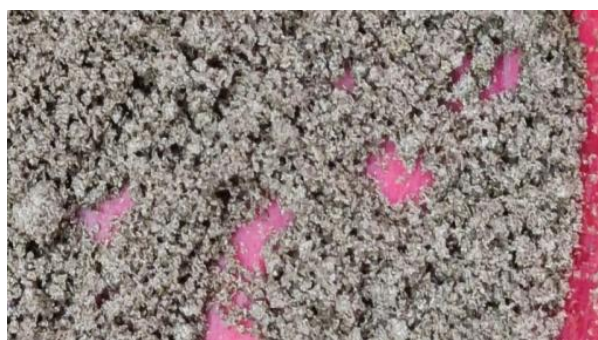
Fig. 2.Chitin, After the process of Deproteinization After the deproteinization (excessive removal of protein ) from the Artemia shells followed by demineralization. The shells which is converted into Chitin polysaccharide
