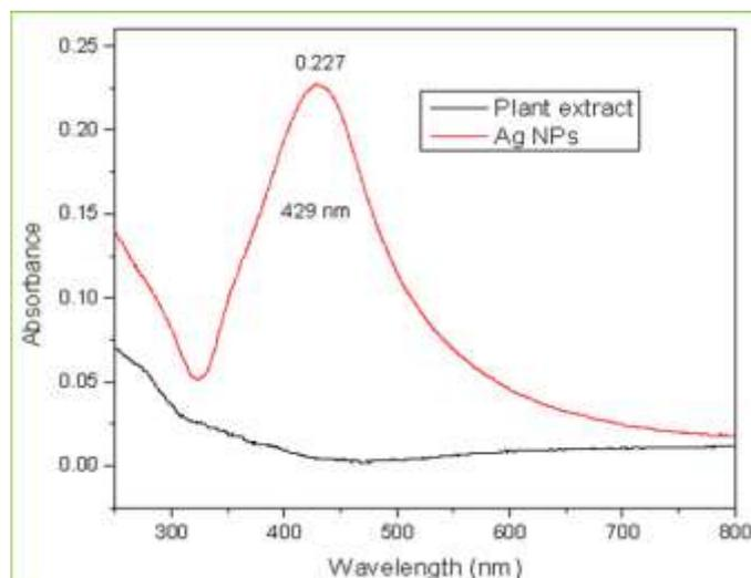
**Fig. 1. UV-Visible Spectrophotometer only one broad peak was obtained at 429 nm, that corresponded to plasmon excitation of silver nanoparticles. Black line indicates plant extract and Red line indicates Ag NPs**
