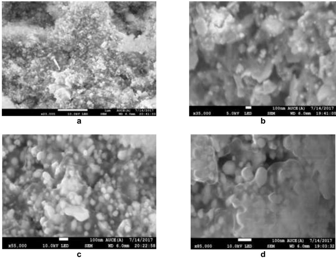
**Fig. 3.** SEM pictures of silver nanoparticles made using *S. siamea* leaf extract at various magnifications, magnifications of X23000, X35000, X55000, and X85000, in that order. The AgNps were found to have an aggregated form and a roughly spherical shape, as seen by the scanning electron microscopy. This indicates that the powder's particles are hexagonal and cubic in shape
