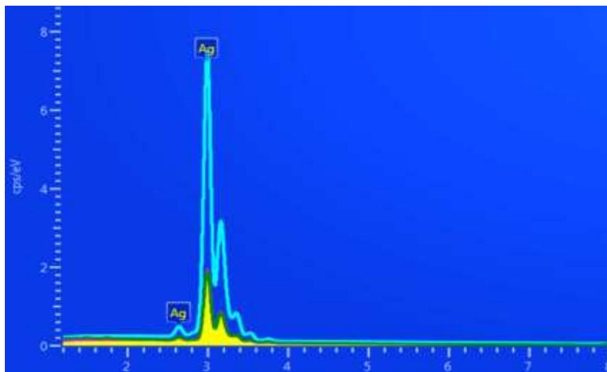
**Fig. 4.** The silver nanoparticles' energy dispersive X-ray spectra revealed a significant silver signal. Figure demonstrates the creation of silver nanoparticles and displays the elemental profile of synthesized nanoparticles made with leaf extracts from *S. siamea*. Because of the silver nanoparticles, Figure also displays increased counts at 3 keV
