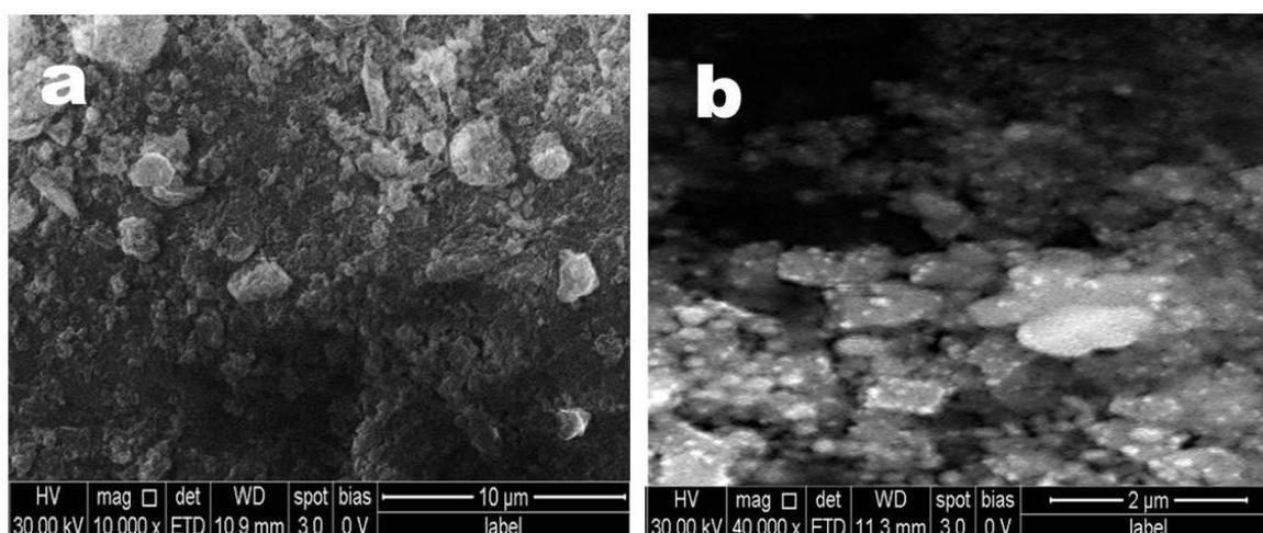
**Fig. 2. Field Emission Scanning Electron Microscopy image of silver nanoparticles (a) and Chitosan coated AgNps (b)**
