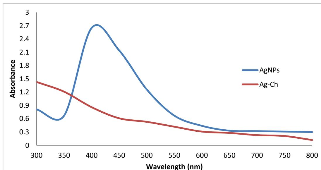
Fig. 1. UV visible spectra of the AgNps and the post reaction mixture AgNps with Chitosan)
