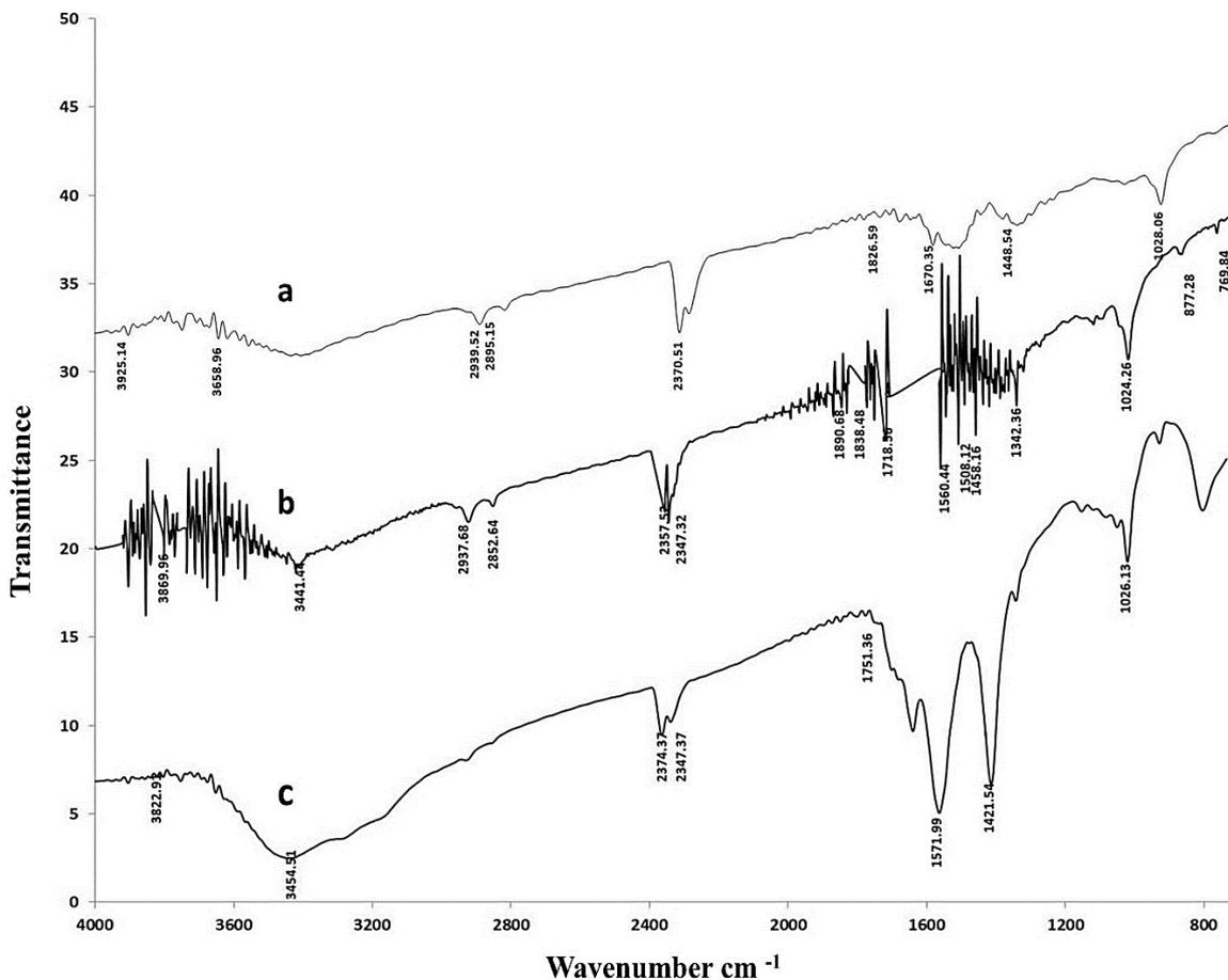
Fig. 3. The FTIR spectra of Ag-Nps (a), Chitosan (b) and Chitosan coated Ag-Nps (c)
